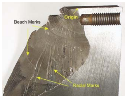
Fig. 8 Beach and radial marks visible on torsional fatigue fracture of a 6 in. diameter 4340 shaft
