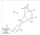
A system for projecting content at an angle to a rear projection screen. The system includes a projector configured for projecting changeable electronic content and a rear projection screen for receiving the projected content at an angle and displaying the projected content.
