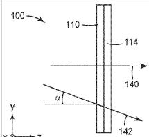
An optical stack including an oriented polymeric multilayer optical film and a non-birefringent optical filter is described. The oriented polymeric multilayer optical film has a first reflection band with a first band edge and the non-birefringent optical filter has a first blocking band. In some cases, the first blocking band contains the first band edge and the first blocking band provides a reduction in variation of a band edge of an overall blocking band of the optical stack.
