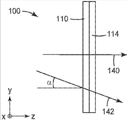
An optical stack including an oriented polymeric multilayer optical film and a non-birefringent optical filter is described. The oriented polymeric multilayer optical film has a first reflection band with a first band edge and the non-birefringent optical filter has a first blocking band. In some cases, the first blocking band contains the first band edge and the first blocking band provides a reduction in variation of a band edge of an overall blocking band of the optical stack.
