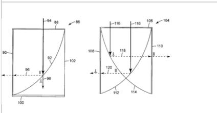
A passive daylight-coupled display having an LCD panel, a diffuser, and a curved reflector behind the LCD panel. For passive backlighting, the diffuser transmits daylight to the reflector, which reflects the daylight to the LCD panel and provides for substantially uniform distribution of the daylight on the LCD panel for backlighting it. A hybrid display includes both a passive backlight and an active backlight for providing backlighting from an active light source.
