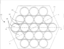
A microfabricated structure to interact with electromagnetic waves, such as a visual display apparatus for positioning movable particles, the structure comprising a substrate containing a plurality of pockets and/or a plurality of posts, and a plurality of optically anisotropic particles placed in the substrate. Pockets are sealable in relation to other pockets and to air, and each pocket being capable of positioning at least one particle.
