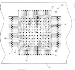
An electronic device adapted for performing molecular biological processes. The device includes a flexible polymeric substrate having a first surface and a second surface. A plurality of microlocations interrupt the first surface, and each of said microlocations include an electrode disposed on the second surface of the flexible substrate. A hydrophilic matrix is positioned on the first surface of the flexible substrate and is capable of electrical contact with the electrode.
