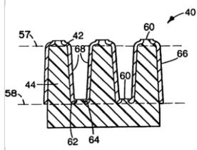
A process for selective metalization for electrically isolating areas of a substrate is disclosed. The process employs placing microridges onto a surface, the microridge protruding from the plane formed by the surface. The surface, including the microridge, is then metalized and a portion of the metalized microridge, beyond the surface plane is removed. This removal process creates electrically isolated areas without affecting the integrity of the substrate.
