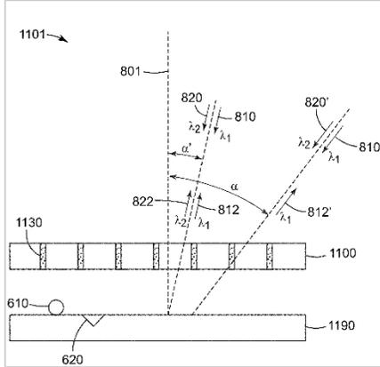
A retroreflective system is disclosed that includes a retroreflective sheet for retroreflecting light, and a light control film disposed on the retroreflective sheet. For a first wavelength, light incident on the light control film at each of a first and second angles of incidence is retroreflected. For a second wavelength, light incident on the light control film at the first, but not the second, angle of incidence is retroreflected.
