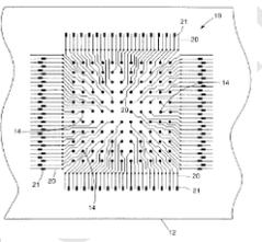
An electronic device adapted for performing molecular biological processes. The device includes a flexible polymeric substrate having a first surface and a second surface. A plurality of microlocations interrupt the first surface, and each of said microlocations include an electrode disposed on the second surface of the flexible substrate. A hydrophilic matrix is positioned on the first surface of the flexible substrate and is capable of electrical contact with the electrode.
