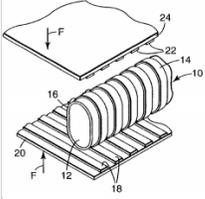
The present invention relates to electronic assemblies which include an elastomeric member made of a cured, room-temperature curable polysiloxane composition. When the assemblies are used to electrically interconnect a first contacting site on a first electronic device to a second contacting site on a second electronic device, the stress-relaxation resistant properties of the elastomer enhance local contact force to maintain a reliable connection.
