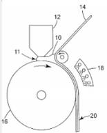
A process for preparing a molded article that includes: (a) bringing a moldable material and an open molding tool comprising a molding surface into line contact with each other to imprint a microfluidic processing architecture pattern onto the moldable material and thereby form a molded article; and (b) separating the molded article from said molding surface. The invention also features various microfluidic processing architecture-bearing, polymeric articles.
