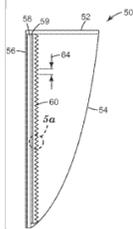
A passive daylight-coupled display having an LCD panel, a diffuser, a turning film behind the LCD panel, and a curved reflector behind the turning film. For passive backlighting, the diffuser transmits daylight to the reflector, which reflects the daylight to the LCD panel through the turning film and provides for substantially uniform distribution of the daylight on the LCD panel for backlighting it. The turning film has prisms with chaos for an improved viewer experience.
