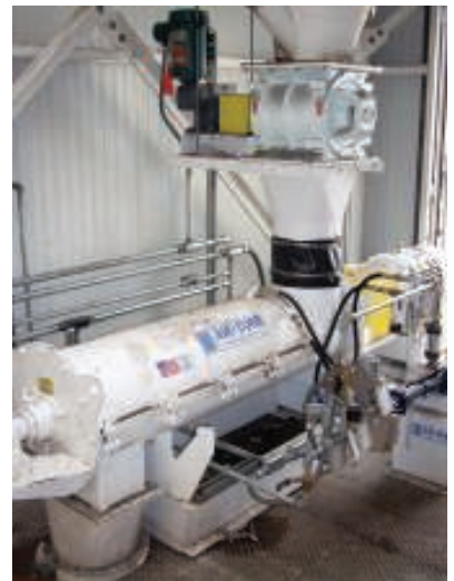
6. Wet and stick. A dust hopper with an agglomeration mixer. Courtesy: Air-Cure Inc.
