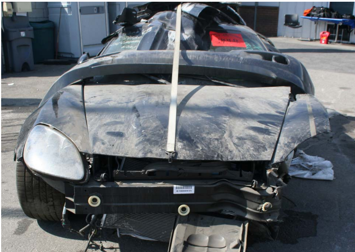
Figure 7. Collision damage resulting in air bag deployment.
