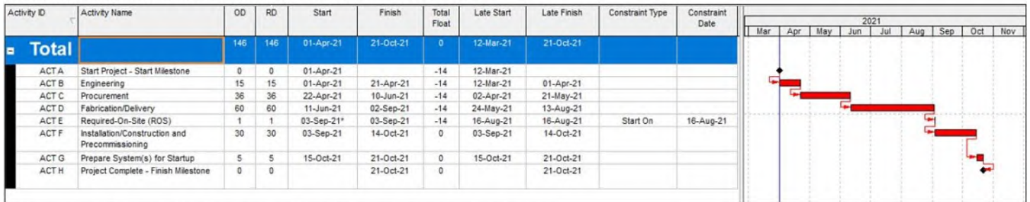
Figure 3-4: Alternative Start Constraint on ACT E
