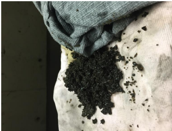
Decomposition of muffler disintegration from oil that is found migrating into the operating valve.
