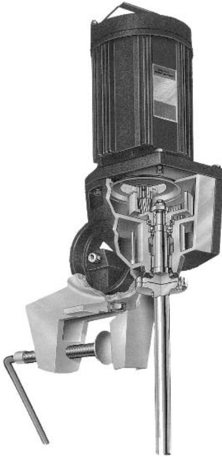
**Figure 21-2** Gear-drive portable mixer. (Courtesy of Lightnin.)
