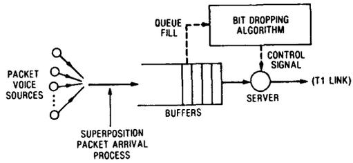
FIGURE 1. PACKET VOICE MULTIPLEXER WITH BIT DROPPING
