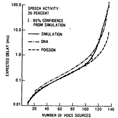
FIGURE 6. EXPECTED DELAY FOR PACKET VOICE MULTIPLEXER
