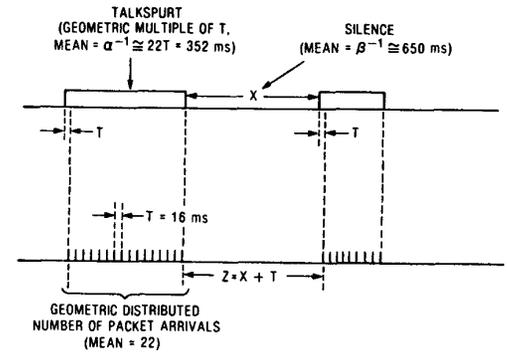
FIGURE 3. PACKET ARRIVAL PROCESS DUE TO ONE VOICE SOURCE
