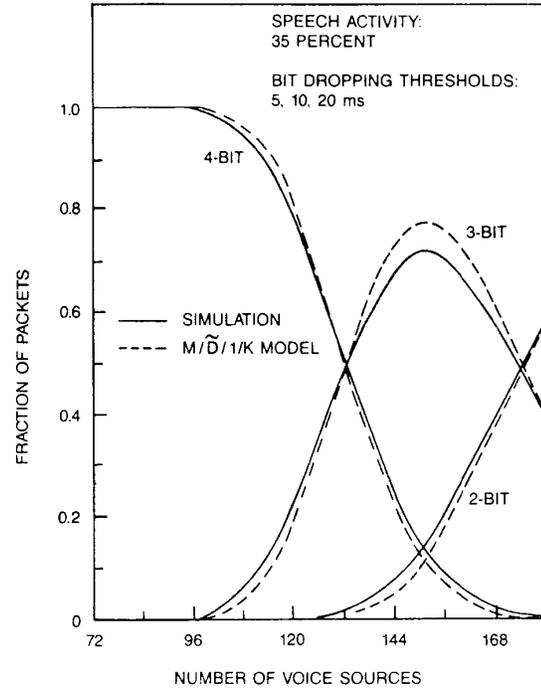
FIGURE 8. FRACTIONS OF PACKETS WITH 4,3,2 BITS PER SAMPLE
