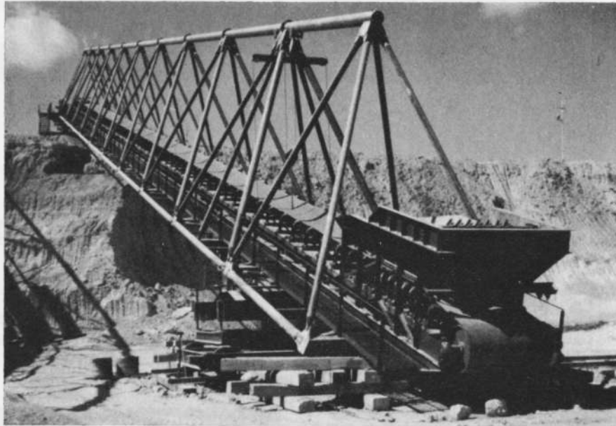
Fig. 3—Bench lift conveyor at Nchanga copper mine in Zambia, central Africa.
