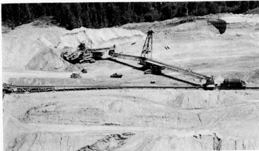
Fig. 2 — Cable reel car, bandwagon, wheel excavator and traveling impact section operated by Washington Irrigation & Development at Centralia, Wash.
