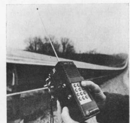
Fig. 13 — Coded radio transmitter at American Electric Power Co.'s James M. Gavin power plant, Cheshire, Ohio.
