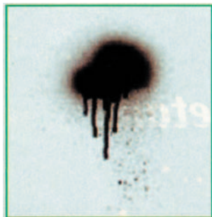
Figure 2. Coarse spray patterns with "hot spots."
