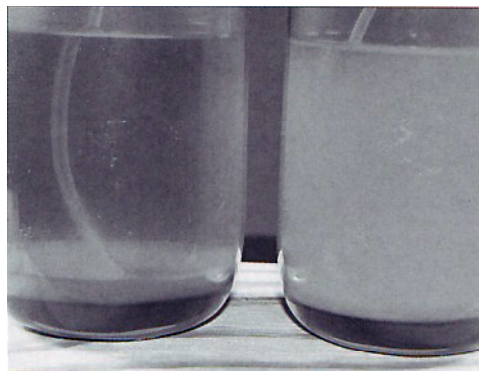
Figure 2: Over time, the glass bottle aerosols clearly indicate which formula is more stable. The bottle on the left, with the dip tube clearly showing, indicates formula instability, with a loss of suspension and the “hard-pack” on the bottom of the vessel. Preferred is the formula that is slow settling, with formula solids still in suspension (and the dip tube obscured).
