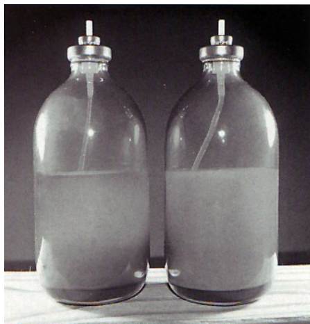
Figure 1: After 30 seconds of shaking, the formula solids remain in suspension and neither dip tube is visible in these glass aerosol bottles. Each contains a different formula, with a different rate of settling for solid ingredients.
