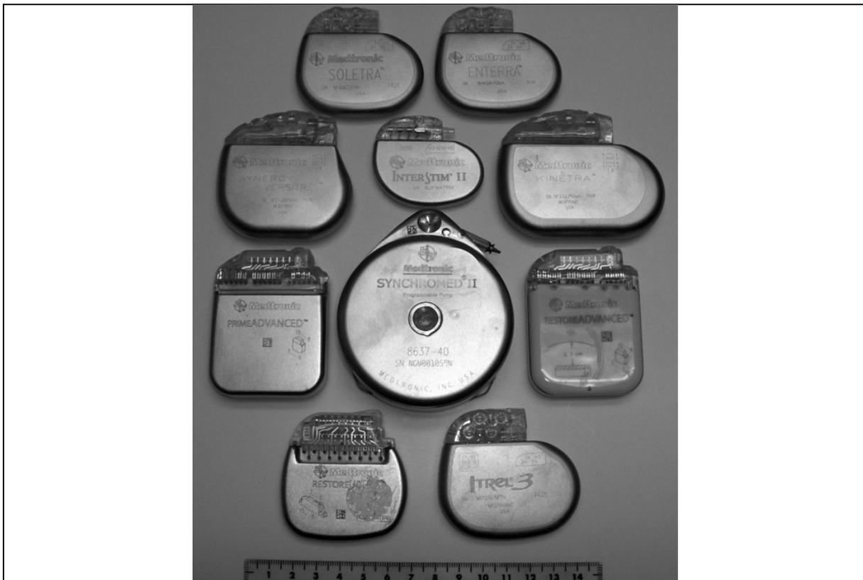
Fig. 2. Medtronic neurostimulation device illustration. Scale is 1.0 cm: At center top down – InterStim II model 3058 and Synchronomed II model 8637-40; Clockwise – Enterra model 3116, Kinetra model 7428, Restore Advanced model 37713, Itriel 3 model 3387, Restore Ultra model 37712, Prime Advanced model 37702, Synergy Versitrel model 7427V, and Soletra model 7426. (Colours are visible in the online version of the article; <http://dx.doi.org/10.3233/XST-2011-0306>)
