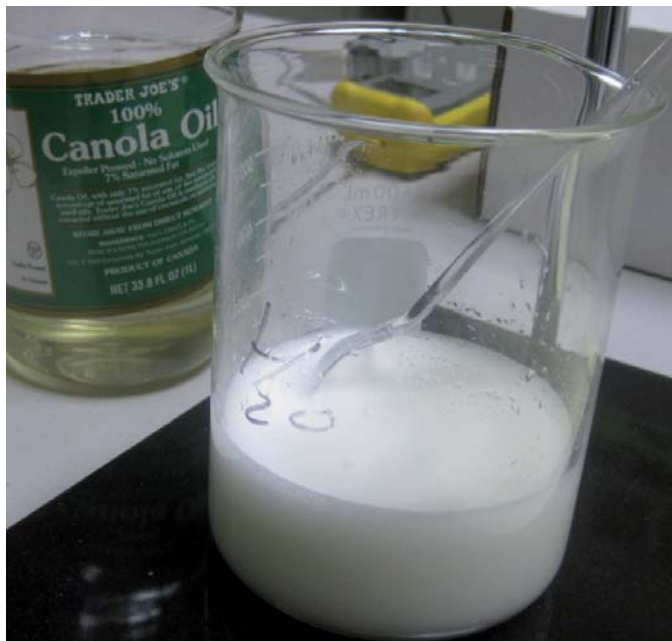
Fig. 7: A close-up view of the 50:50 experimental Jojoba-water emulsion
