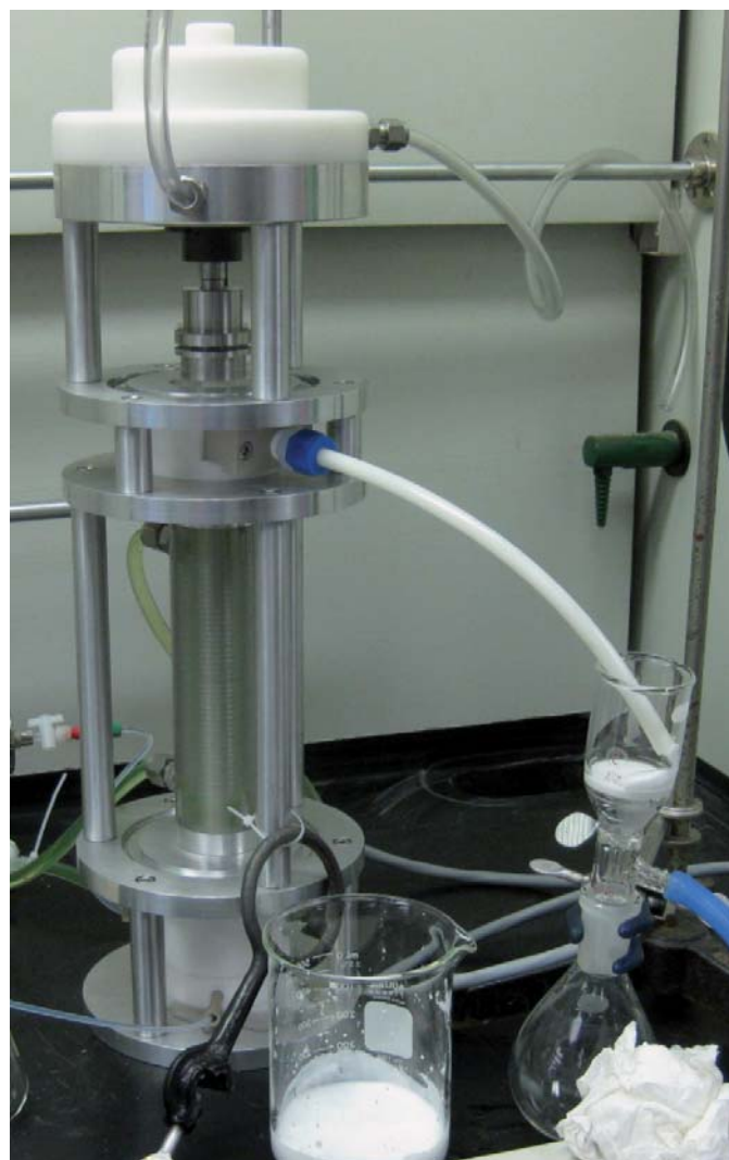
Fig. 6: A Holl-Ergatron™ emulsicator during production of a 50:50% experimental Jojoba-water emulsion
