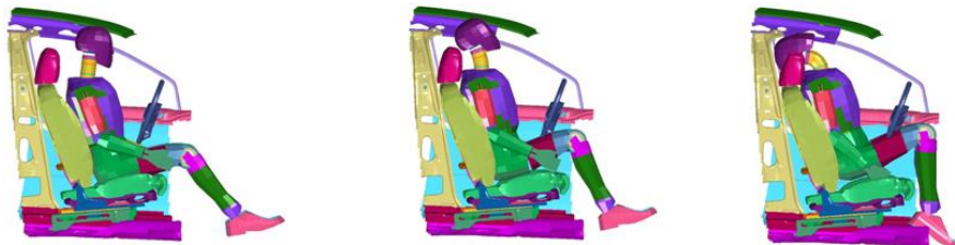
Driver 50th percentile ATD, Rigid Seat, Rear Impact
