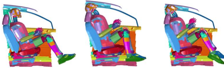
Driver 95th percentile ATD, Rigid Seat, Rear Impact
