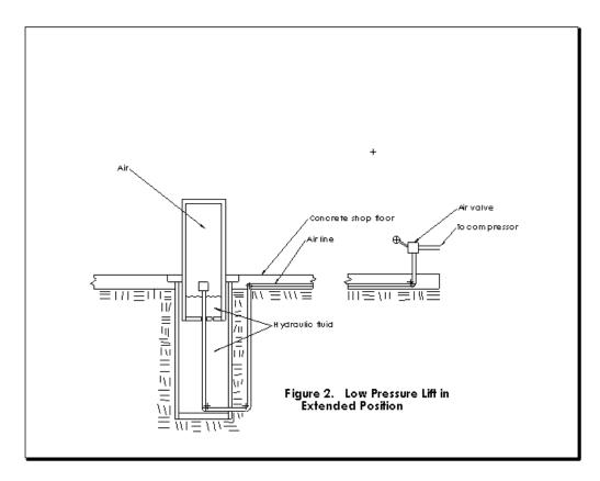
Lifts with this same general configuration have been sold and installed in repair shops for over fifty years. Some of these lifts have a mechanical lock system (not shown in the figures above) which provide a secondary means of supporting the load when the lift is extended. Although these locks have been available for over fifty years, they have been optional devices on most lifts, and many of the older lifts found in repair shops around the United States do not have them.
