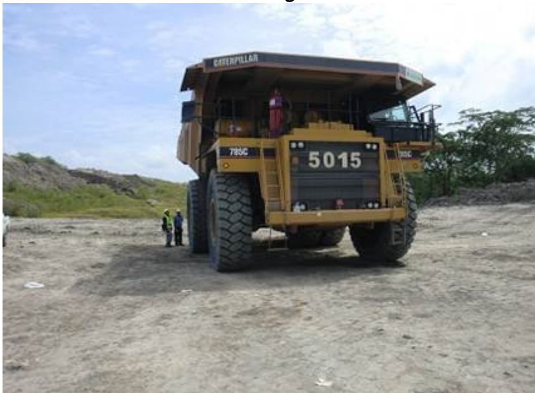
Figure 1: 33.00R51 OTR Tires on CAT 785C
